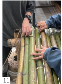
Fig 11. | Work photos of bamboo prop construction, utilizing traditional techniques such as hemp rope or reinforcement fixing, and refining the structure to fit onto a wooden frame for easier transportation to the theatre.
